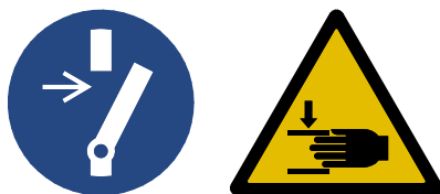
6697 – Inspection cover/inspection door: “Disconnect completely before working”, “Warning of risk of crushing”
